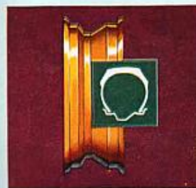
Safety Rim Wheel for your protection in case a tire blows out—holds tire firmly in place.
