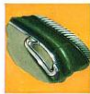
Assist handles, rigid mounted on front seat back, are a safety and convenience feature.
