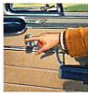
Electric Window Lifts, with separate motor on each window, available at extra cost.
