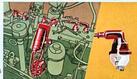
Waterproof Ignition for sure starts in damp or rainy weather. Spark Plugs, Coil, Wiring, and Distributor are waterproofed.
